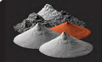
GKN's material capabilities range from high performance gas atomized powders to high productivity water atomized powders.
