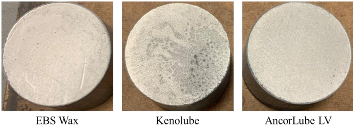
Figure 10: Surface condition of sintered slugs made from FC-0208 premix with 0.6% admixed lubricant
