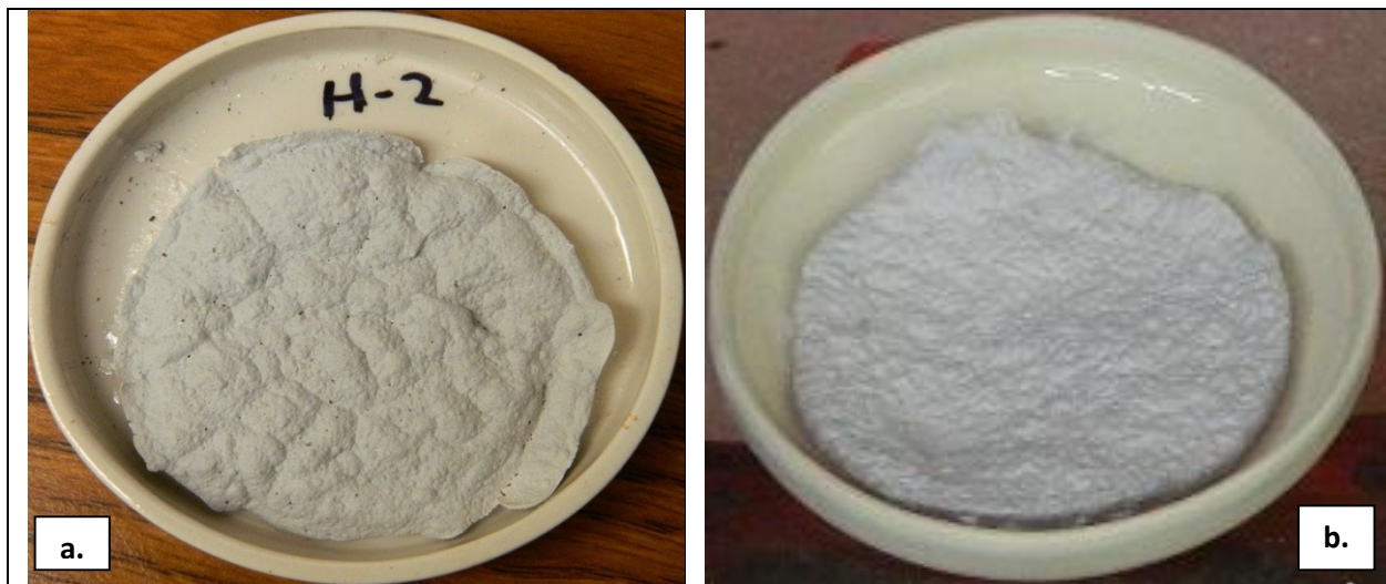
Fig. 3. Appearance of the Insulation Film “H” (a) and the Insulation Film “T” (b) After Heat Treatment, being performed at 870°C (1600°F) in Ambient Air Atmosphere (Batch Furnace) Conditions.
