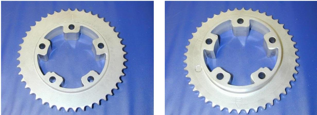
**Figure 4:** Photograph of VVT part showing major short hub OD on left and major long hub on right
