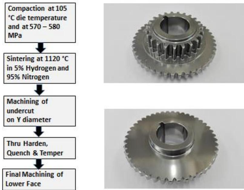
**Figure 4:** Processing Sequence for the prototype production of the crank sprocket
