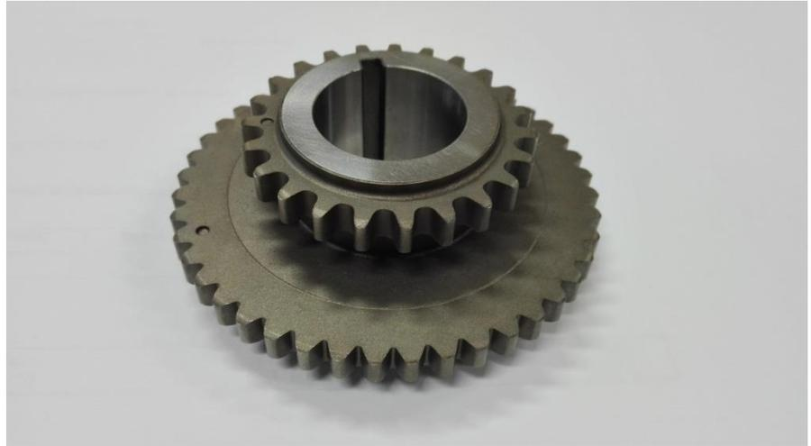
**Figure 3:** Photograph of finished crank sprocket evaluated in this study
