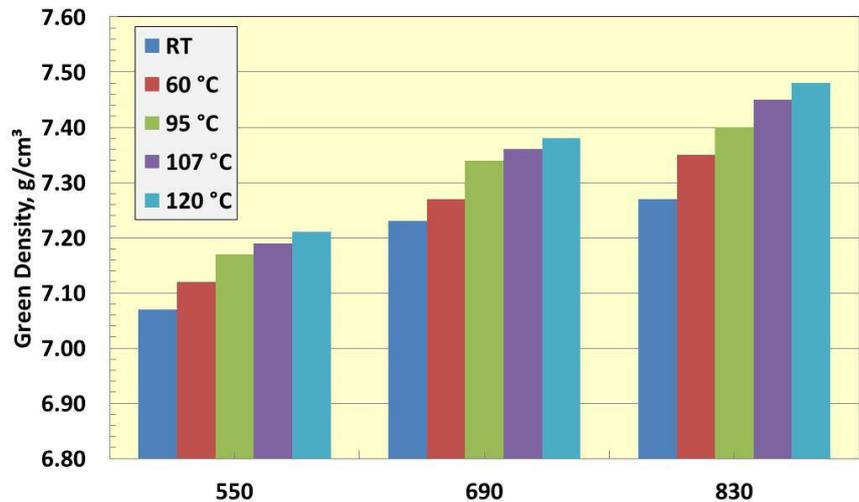
**Figure 1:** Effect of compaction pressure and die temperature on green density
