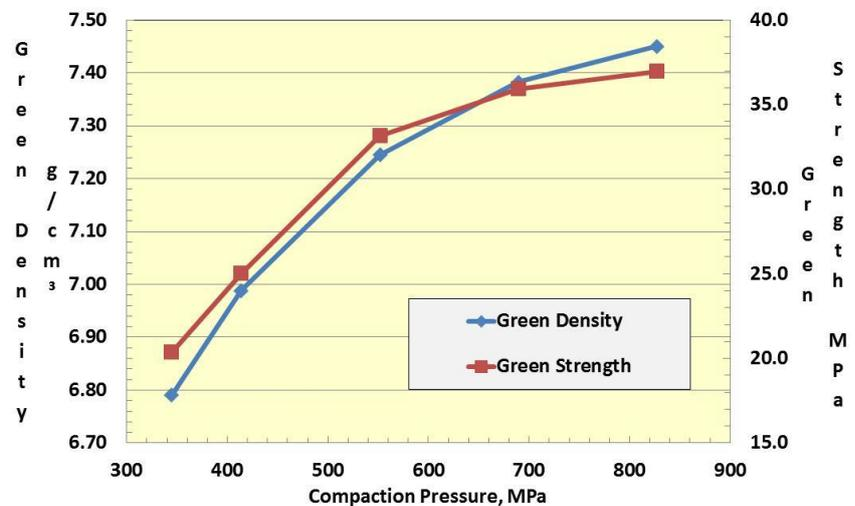
**Figure 2:** Green density and green strength of AncorMax 225 FLN2-4405
