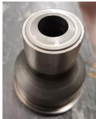
Figure 4: Punch geometry for production trial at Phoenix Sintered Metals
