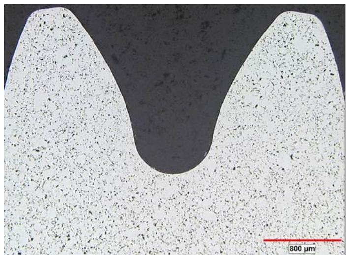
**Figure 5:** Photomicrograph of 0.80 mm module gear demonstrating the uniformity of density from body of gear to the apex of gear tooth
