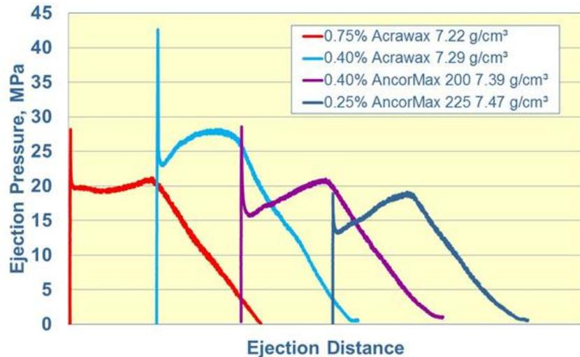
**Figure 6:** Ejection characteristics of a common lubricant compared to the AncorMax 225 lubricant system, all samples compacted at 760 MPa. The Acrawax® samples were compacted at 25°C, the AncorMax 200 compacted at 93°C, and the AncorMax 225 sample compacted at 105°C.
