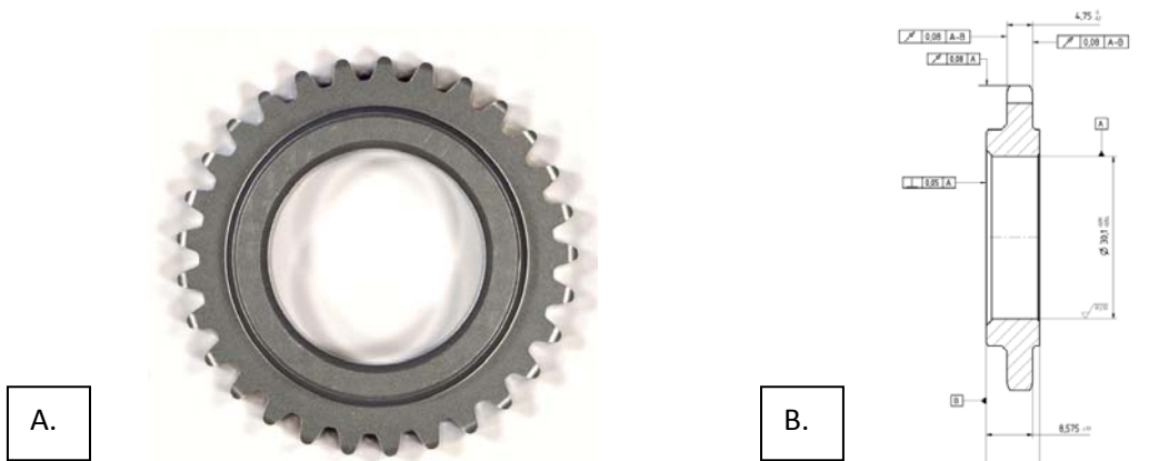
Figure 1: (A) Image of serial production sprocket having a nominal ID of 30.1 mm and overall OD of 56.64 mm; (B) cross-sectional schematic.
