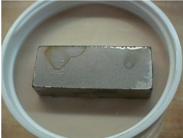
Figure 8 (a): SS-316N1 test bar after ½ h Class B = 0-1% rust
