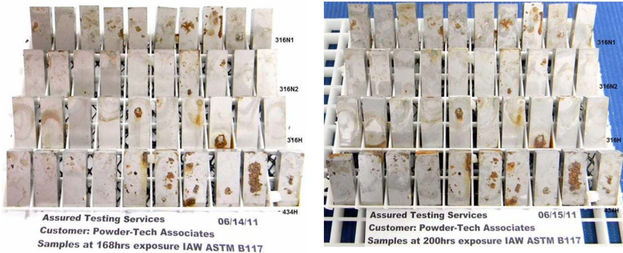
Figure 12: Photographs of the various test bars after 168 h and 200 h of salt spray exposure.
