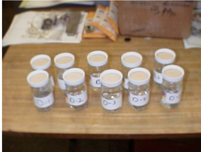
Figure 1: Example of the experimental set-up for immersion testing in accordance with ASTM B895).
