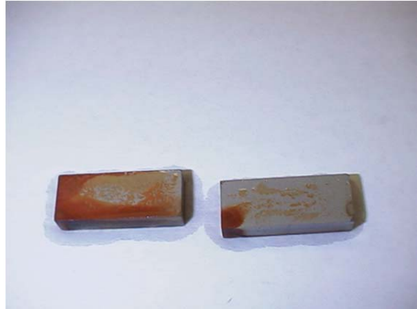
Figure 8 (b): SS-316N2 test bars after 96 h On left Class D = >25% rust On right Class C= 1-25% rust
