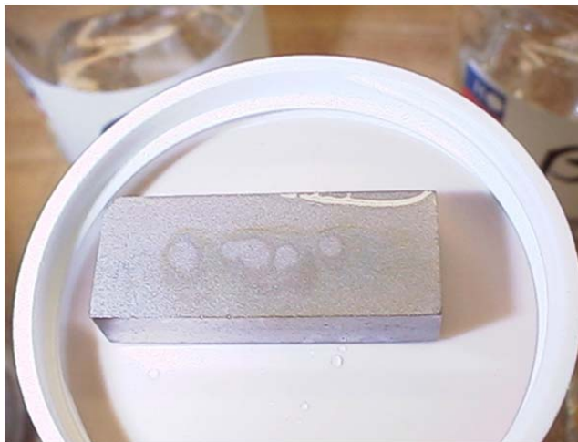
Figure 7 (a): SS-434H test bar after ½ h Class B = 0-1% rust
