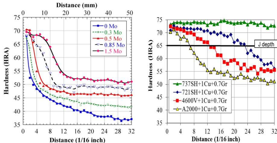
Figure 1: Jominy end-quench hardness profiles of PM steels at 7.0 g/cm<sup>3</sup> with (a) different levels of Mo content and 0.6 w/o graphite; and (b) typical sinter-hardening alloy compositions readily available to the market.
