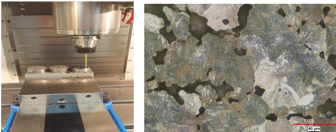
Figure 2: a) Drilling set up with aluminum fixture; b) Nital etched microstructure. FC-0208.
