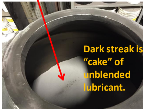
Figure 12: Upset condition measured during dynamic testing showing effusivity decrease (top) due to “cake” of lubricant.
