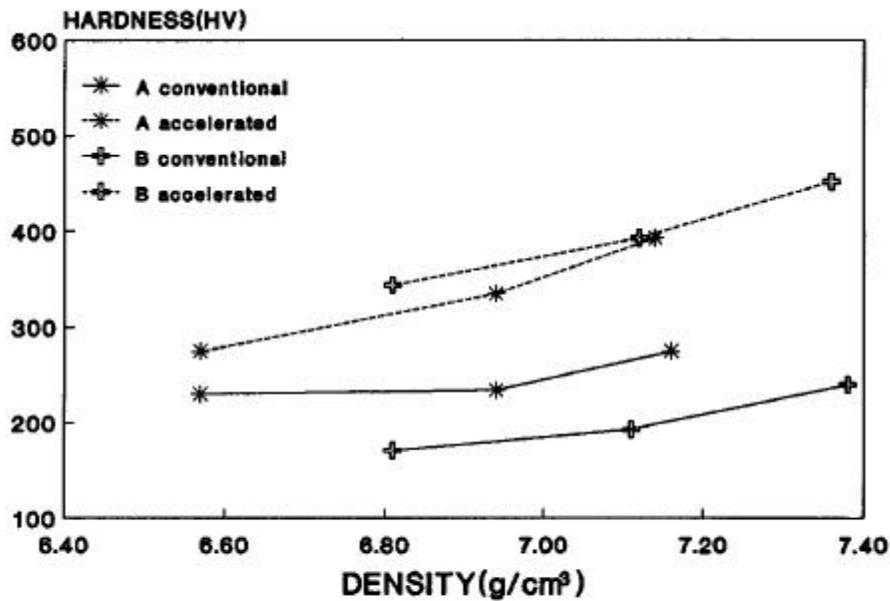
Figure 7: The effect of sintered density and cooling rate on the apparent hardness of materials A and B.
