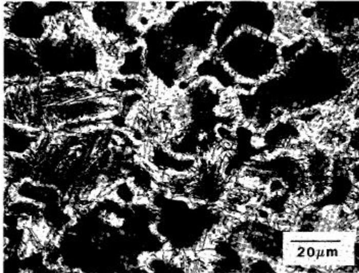
**Figure 3:** Photomicrograph of material B following conventional cooling from the sintering temperature. Etched with a combination of 2% nital/4% picral. Original magnification 750X.
