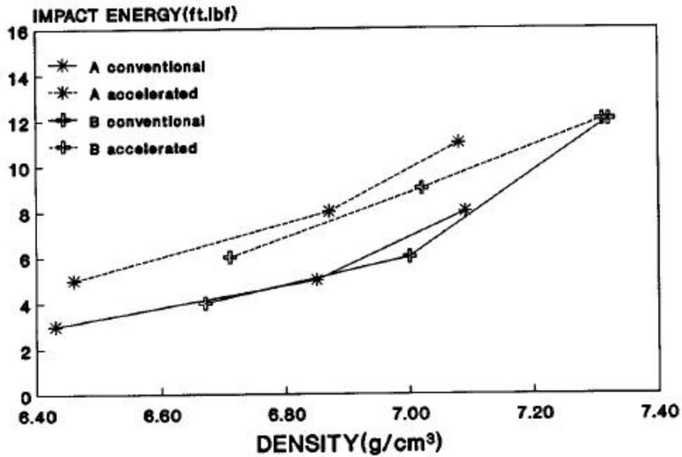
Figure 6: The effect of sintered density and cooling rate on the unnotched Charpy impact energy of materials A and B.
