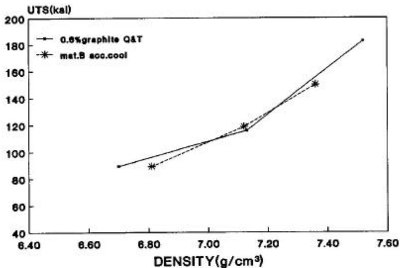
Figure 8: Comparison between the ultimate tensile strength of quenched and tempered Ancorsteel 85 HP, 0.6% graphite, and material B following accelerated cooling from the sintering temperature.
