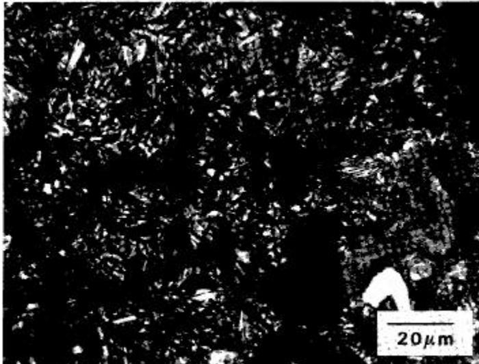
**Figure 4:** Photomicrograph of material B following accelerated cooling from the sintering temperature. Etched with a combination of 2% nital/4% picral. Original magnification 750X.
