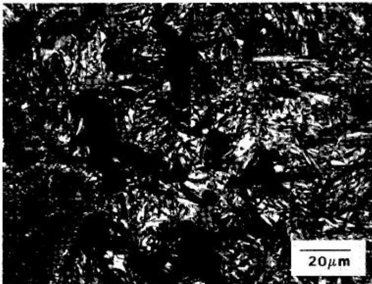
**Figure 2:** Photomicrograph of material A following accelerated cooling from the sintering temperature. Etched with a combination of 2% nital/4% picra
