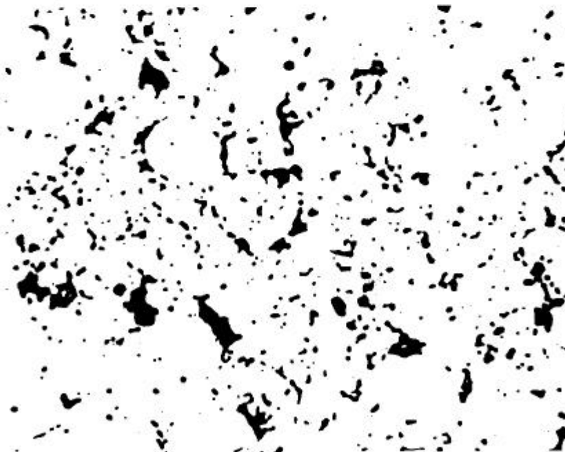
Figure 4 - Same as Figure 3 but with 1% copper addition. Larger pores are readily evidenced.
