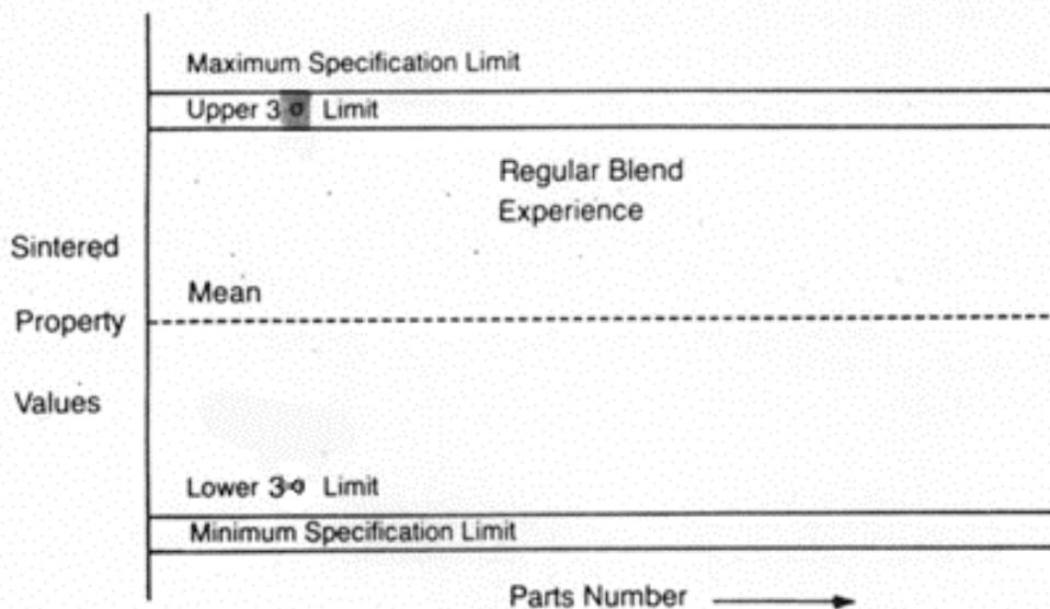
Figure 5 Control Chart Schematic of a Regular Blend Property
