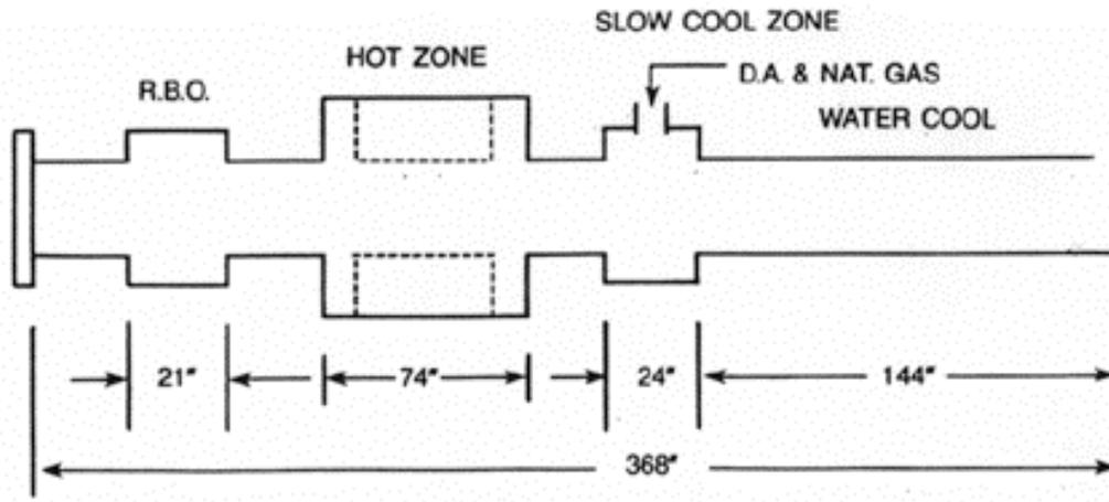
Figure 1 - Plan View of Sintering Furnace
