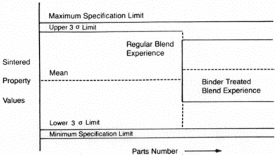
Figure 6 Control Chart Schematic Comparing Regular and Binder Treated Blends
