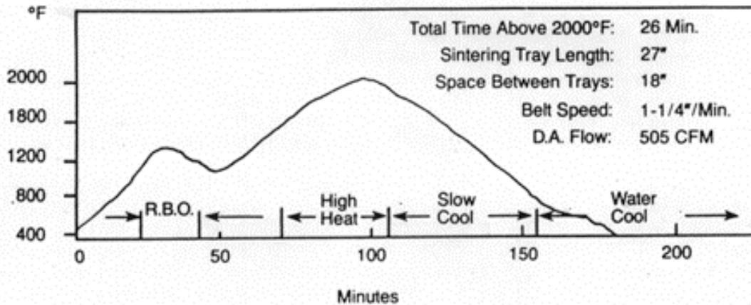
Figure 2 - Furnace Temperature Profile and Sintering Details
