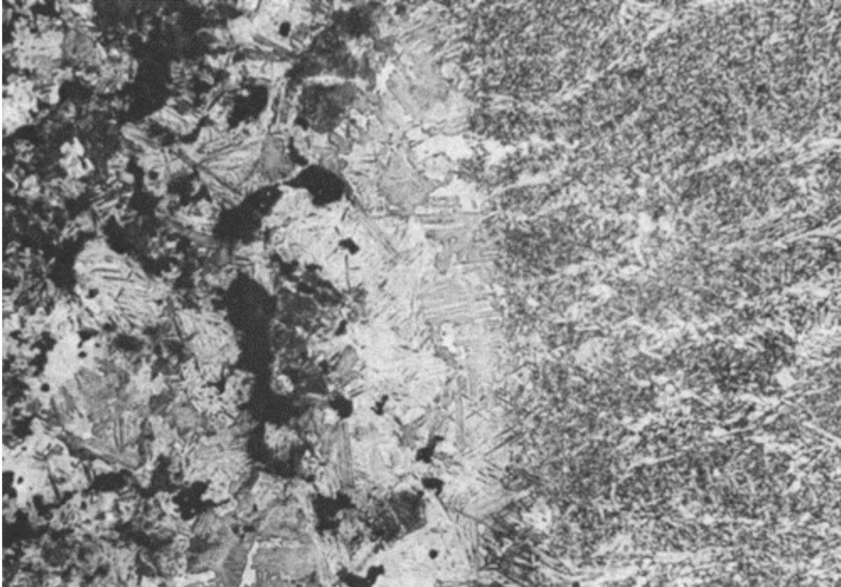
**Figure 1: Weld interface showing P/M martensitic structure (left) and low-carbon filler metal with dendritic structure (right).200X**
