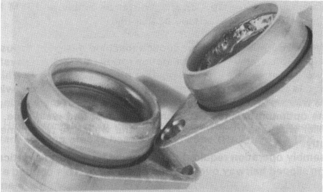
**Figure 3: Examples indicating acceptable weldment (left) and extreme porosity (right).**
