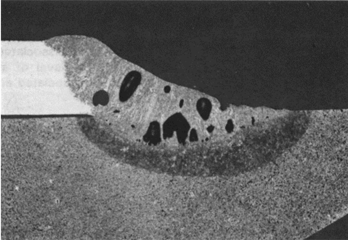
Figure 4a: High percentage of interstitial gases resulted in extreme porosity. Dark etching area is heat affected zone (HAZ).
