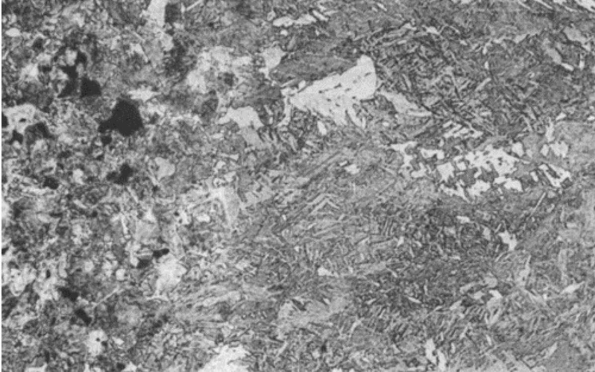
**Figure 2: Martensitic wrought alloy steel (right) joined to low-carbon P/M steel (left). 200X**
