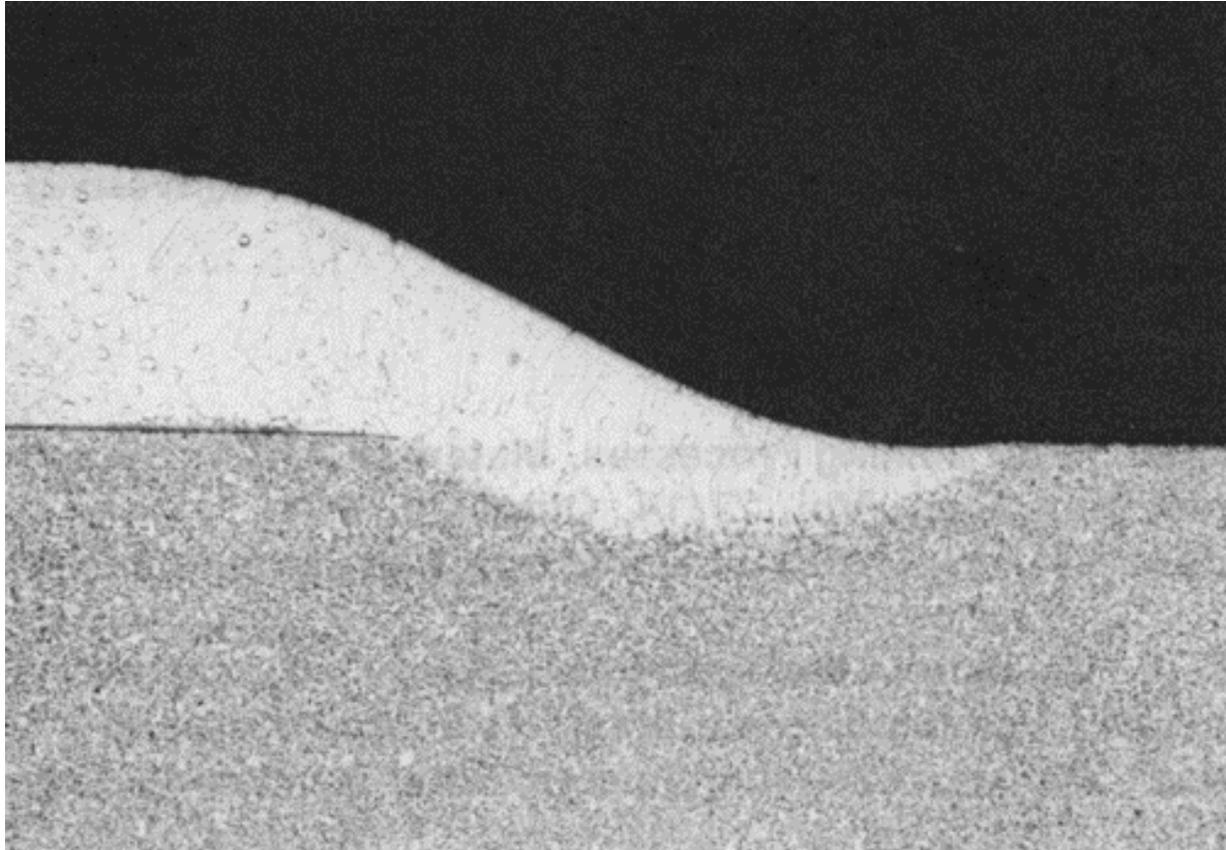
**Figure 5a: Illustrates a sound weldment to a hydrogen sintered bushing. 12X**
