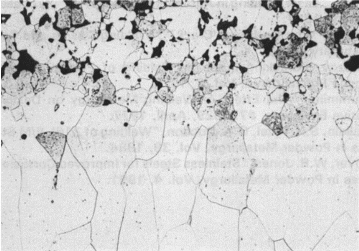
**Figure 5b: High magnification of etched weldment verifies ferritic microstructure. 200X**
