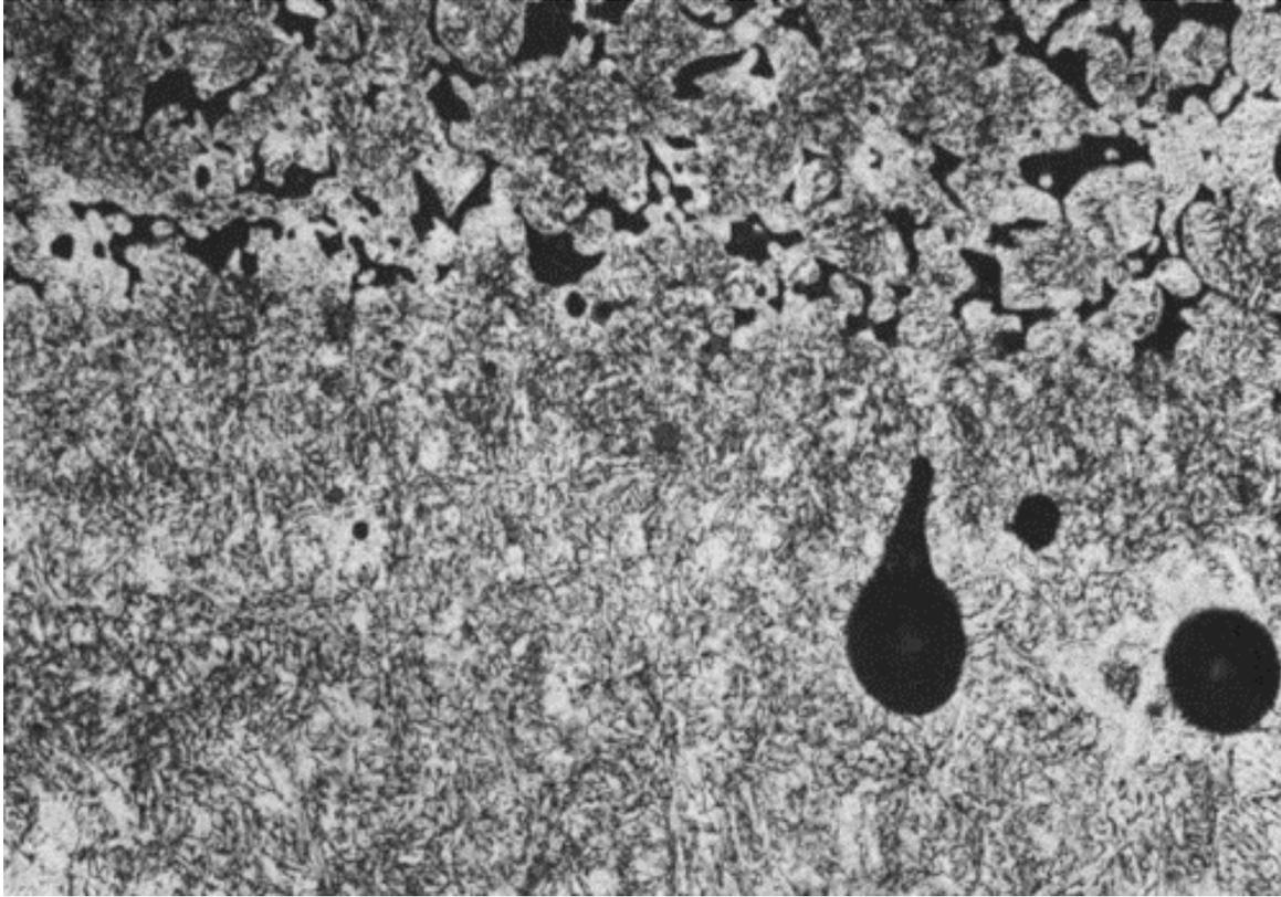
**Figure 4b: Higher magnification indicates martensitic transformation in HAZ and P/M part. 200X**
