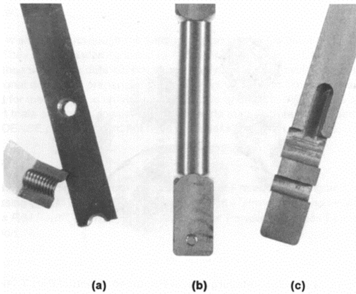
Figure 13: Examples of Green Machined ANCORDERSE Samples
