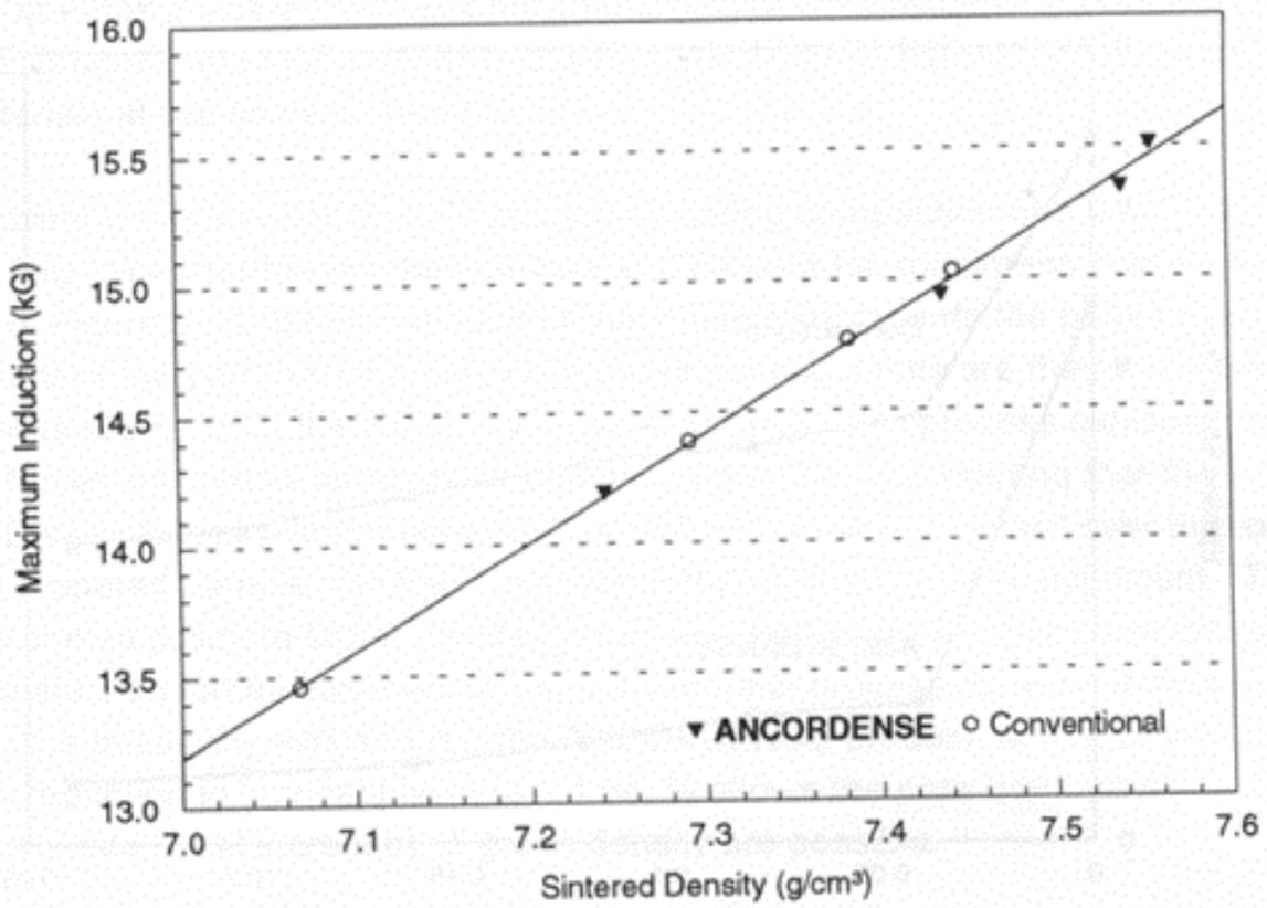
Figure 11: The effect of Density of Ancorsteel 45P on Maximum Induction Measured at 30 Oe(Sintered at 2300°F for 30 minutes in a 100% H<sub>2</sub> atmosphere)
