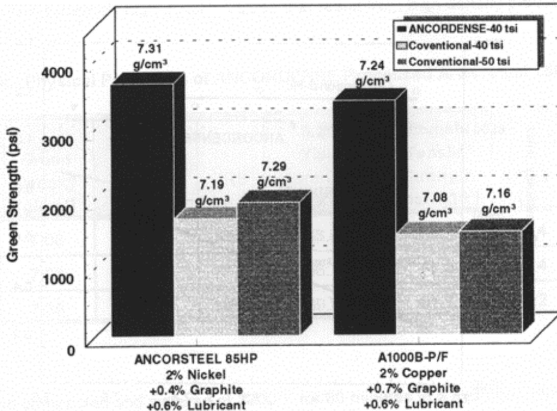
Figure 12: Green Strength for Several Premix Compositions Compacted Utilizing ANCORDENSE and Conventional Techniques
