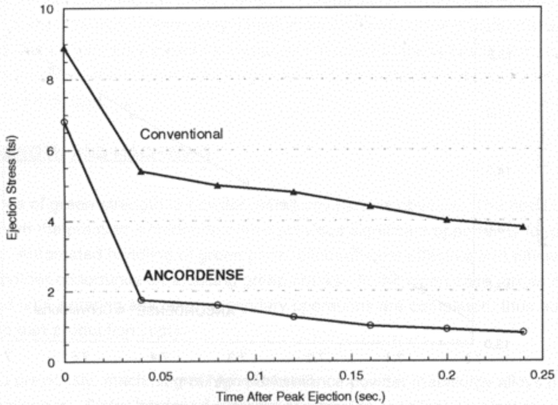
Figure 9: Ejection Stresses for ANCORDENSE and Conventionally Processed Premixes of Distaloy 4800+0.6% Graphite+0.6% lubricant (0.4"x0.4"x2.5" bar)
