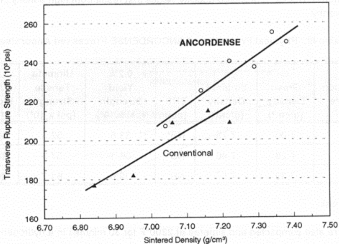
**Figure 8: Transverse Rupture Strength for ANCORDERSE and Conventionally Processed Premixes of Distaloy 4800+0.6% Graphite +0.6% Lubricant (Sintered at 2050°F for 30 minutes in a 75% H<sub>2</sub>/25% N<sub>2</sub> atmosphere)**
