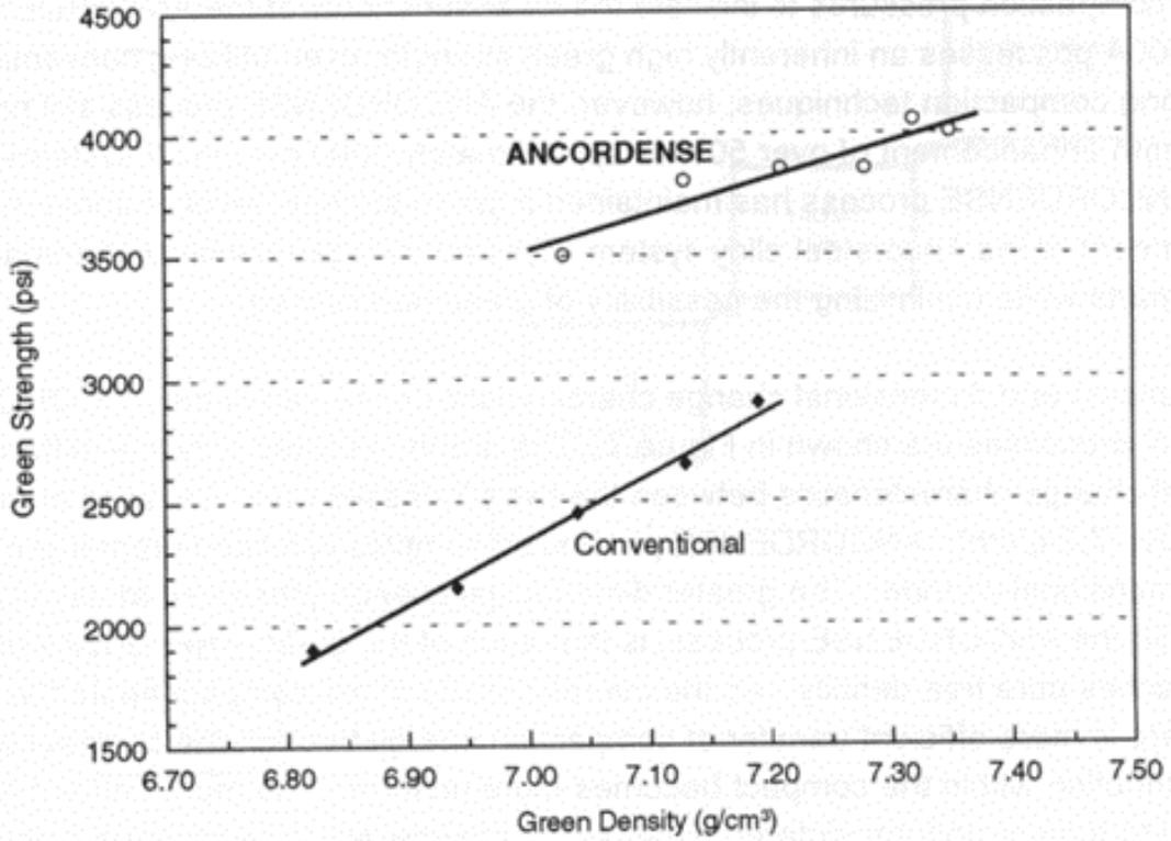
Figure 6: Green Strength of Distaloy 4800+0.6% Graphite+0.6% Lubricant Compacted Conventionally and with the ANCORDERSE Process
