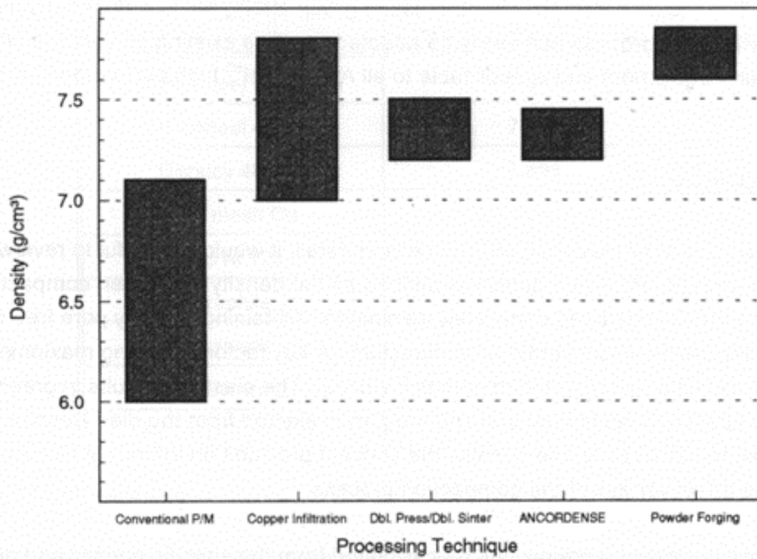
Figure 1. Typical Density Ranges for Several Common Powder Metallurgy Processes
