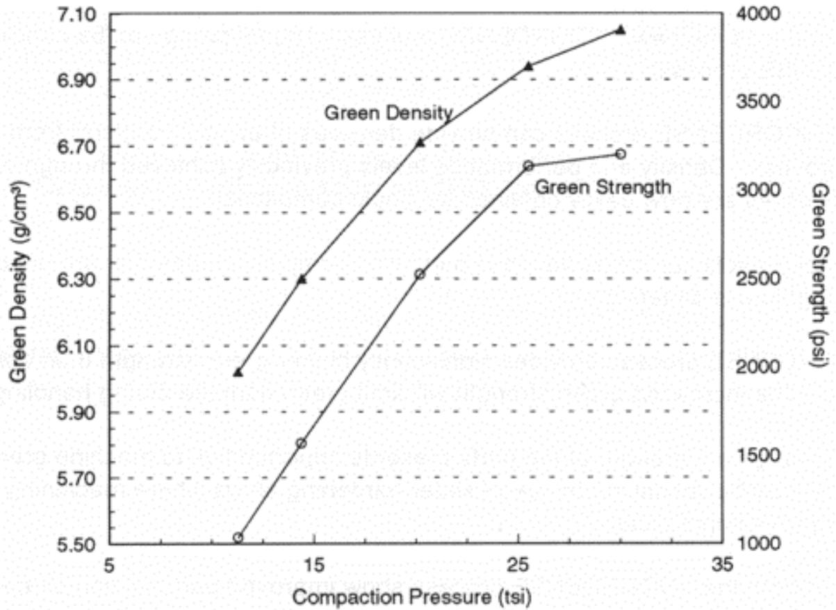
Figure 14: The Effect of ANCORDENSE Processing at Low Compaction Pressures (Acorsteel 1000B P/F+2.0% Cu+0.5% MnS+0.7% Graphite+0.75% Lubricant)
