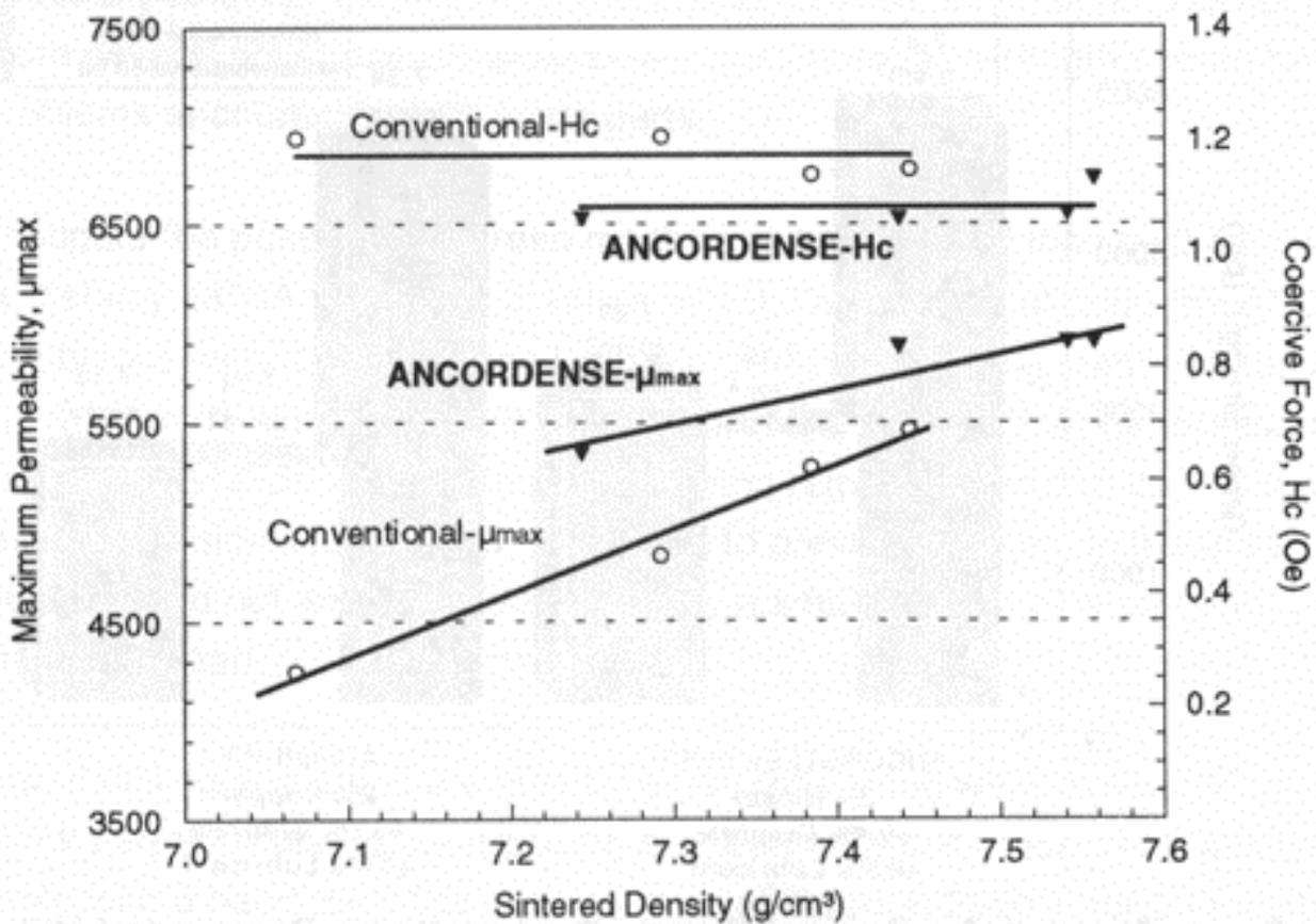
Figure 10: Magnetic Properties for ANCORDENSE and Conventionally Processed Ancorsteel 45P (Sintered at 2300°F for 30 minutes in a 100% H<sub>2</sub> atmosphere)
