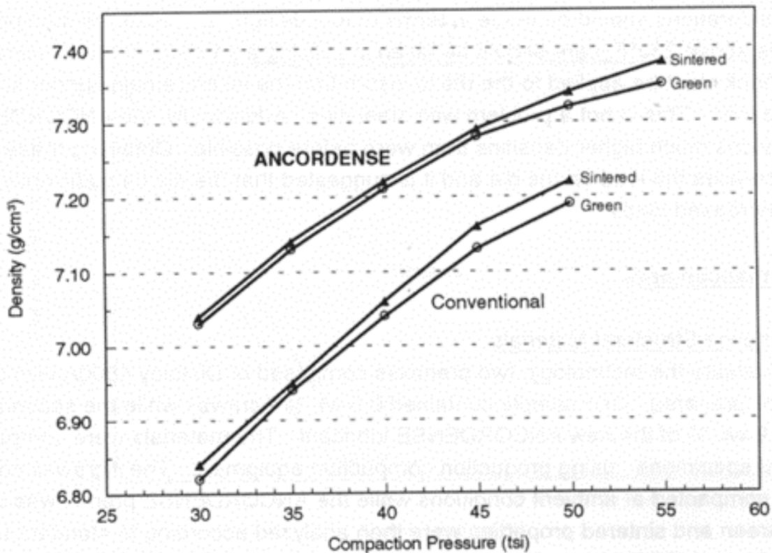
Figure 5: Green and Sintered Density for ANCORDERSE and Conventionally Compacted Premixes of Distaloy 4800A+0.6% Lubricant (Sintered at  $2050^{\circ}\text{F}$  for 30 minutes in a 75%  $\text{H}_2$ /25%  $\text{N}_2$  atmosphere)
