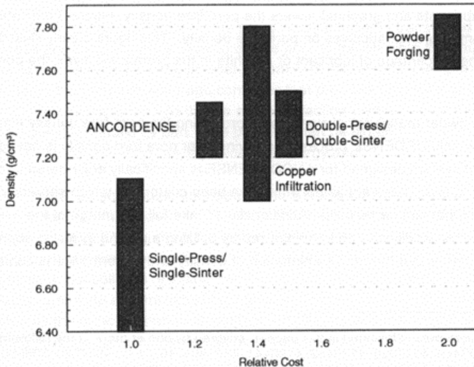
**Figure 2. The Relative Cost and Density Ranges for Various Powder Metallurgy Processes**
