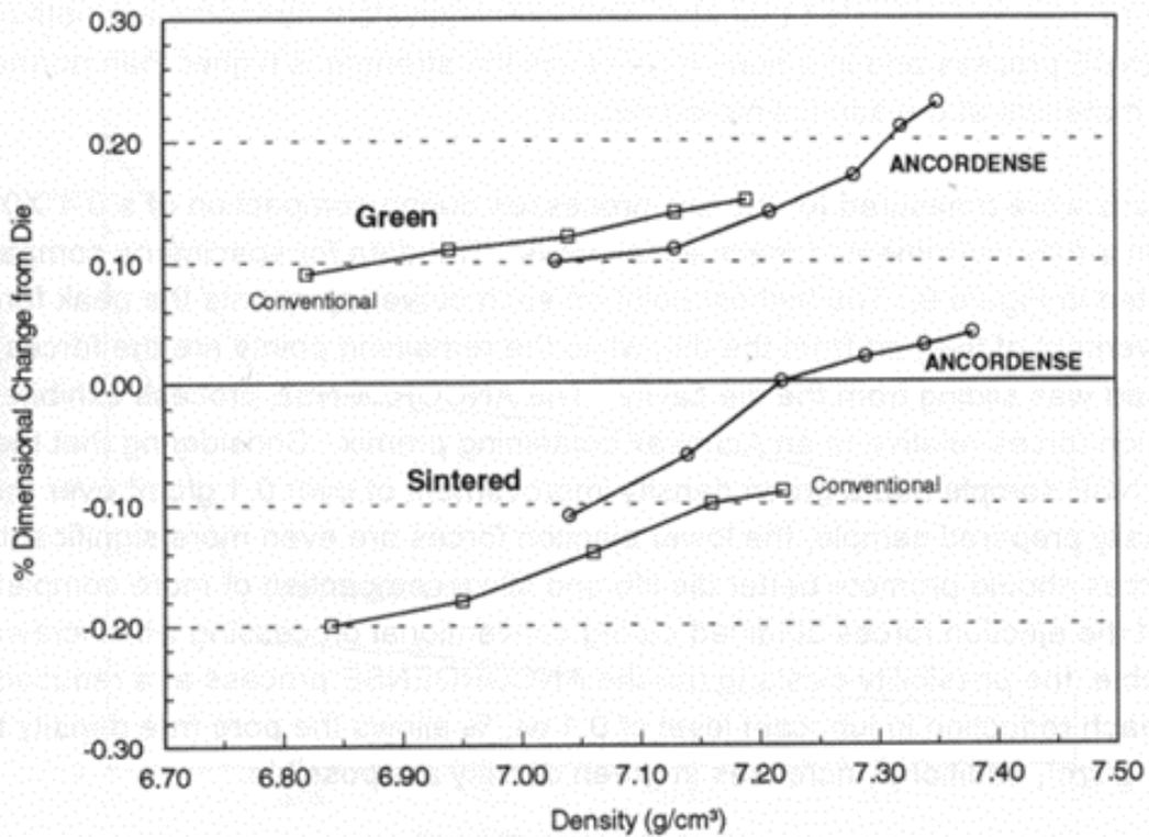
Figure 7: Dimensional Change From Die Size for Distaloy 4800A+0.6% Graphite+0.6% Lubricant Compacted Conventionally and with the ANCORDERSE Process (Sintered at 2050°F for 30 minutes in a 75% H<sub>2</sub>/25% N<sub>2</sub> atmosphere)
