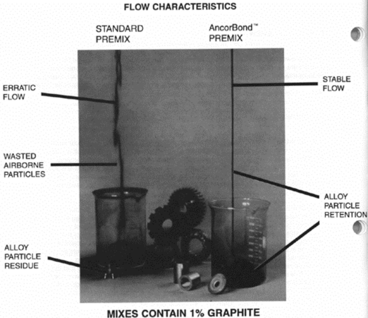
**Figure 1: Flow/fill characteristics of conventional and ANCORBOND premixes. ANCORBOND processing improves flow rate, fill uniformity and reduces dusting/segregation.**
