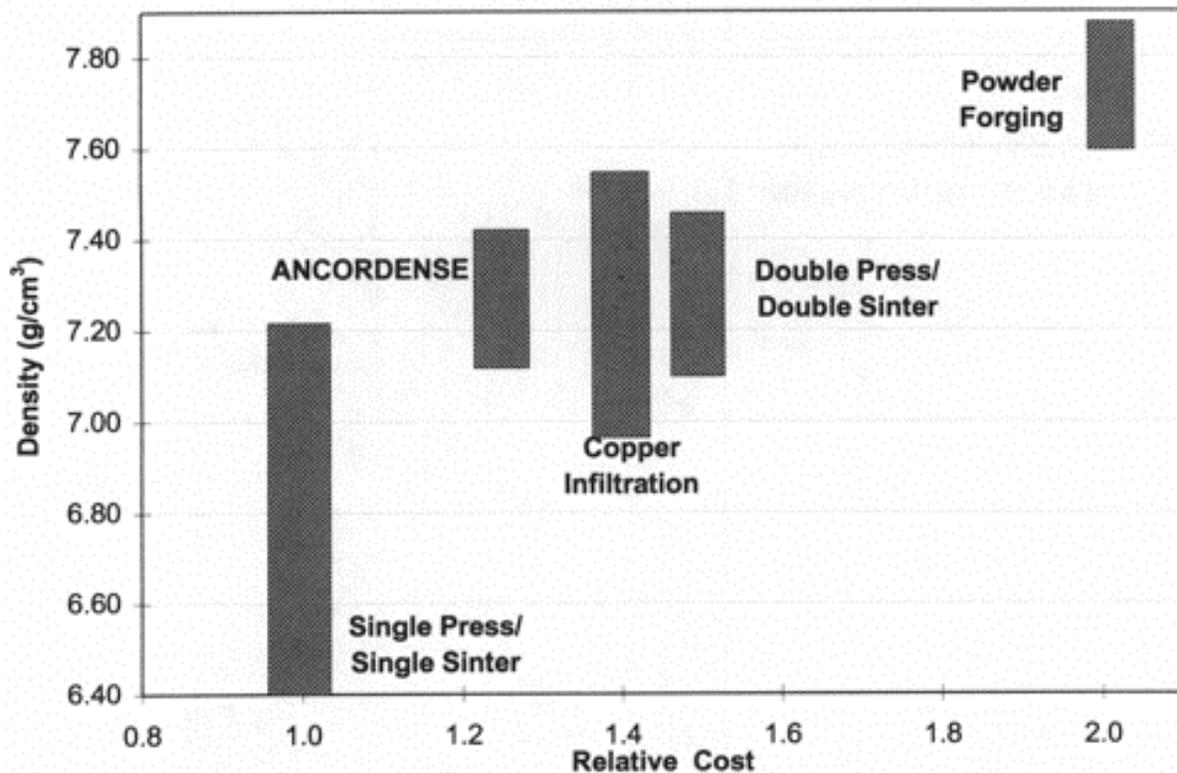
**Figure 3: The Relative Cost And Density Ranges For Various Powder Metallurgy Processes.**
