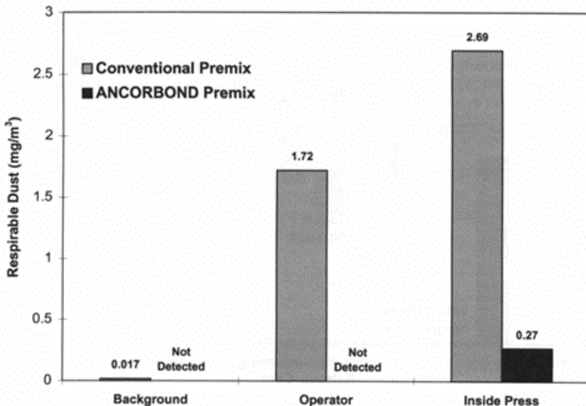
Figure 2: Respirable Dust In Work Area for a Conventional Premix and an ANCORBOND Premix.
