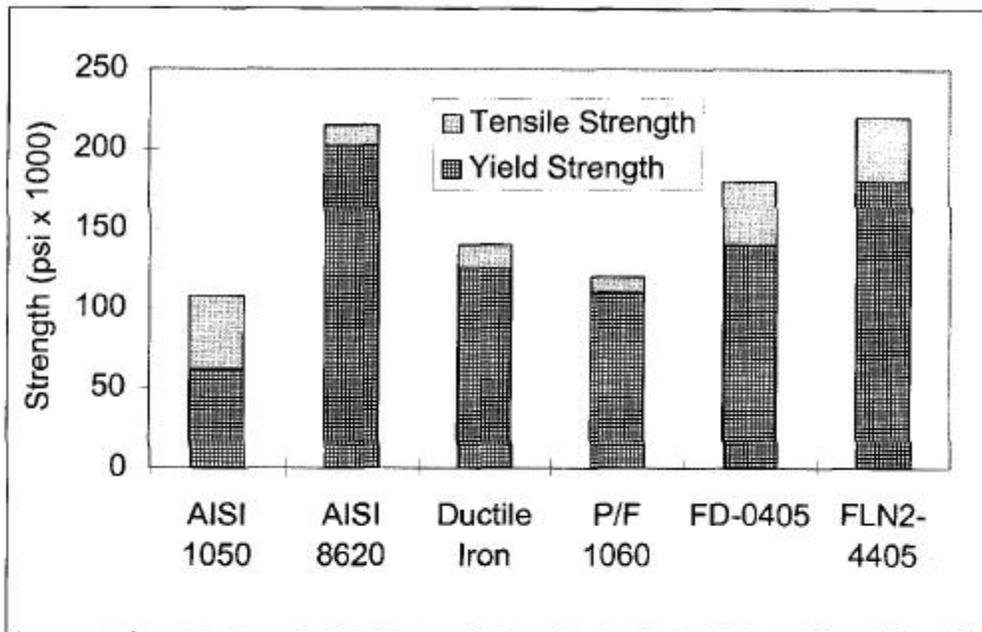
Figure 3: Mechanical properties of wrought and ANCORDENSE materials in heated treated condition.
