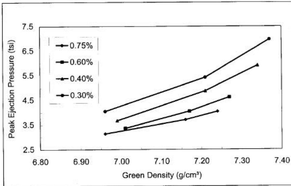
**Figure 5: Effects of reduced lubricant levels on the ejection forces of conventionally compacted materials. The lubricant used was Acrawax.**
