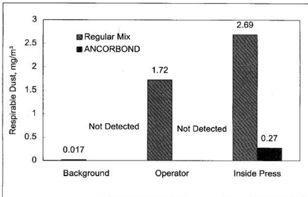
Figure 1: Respirable dust in work area for a conventional premix and ANCORBOND premix.
