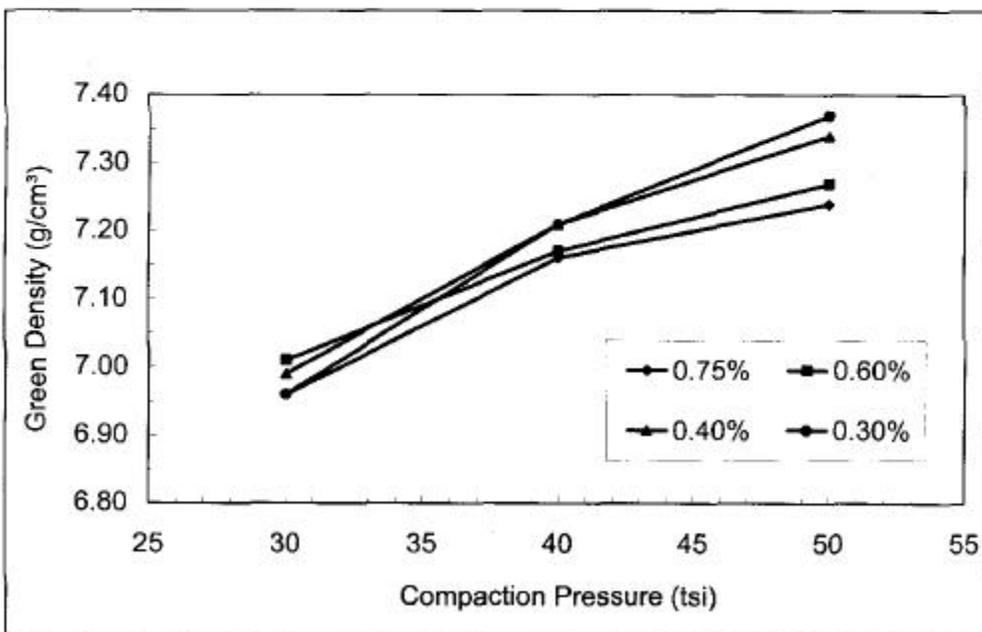
Figure 4: Effects of reduced lubricant levels on the green density of conventionally compacted premixes. The lubricant used was Acrawax.
