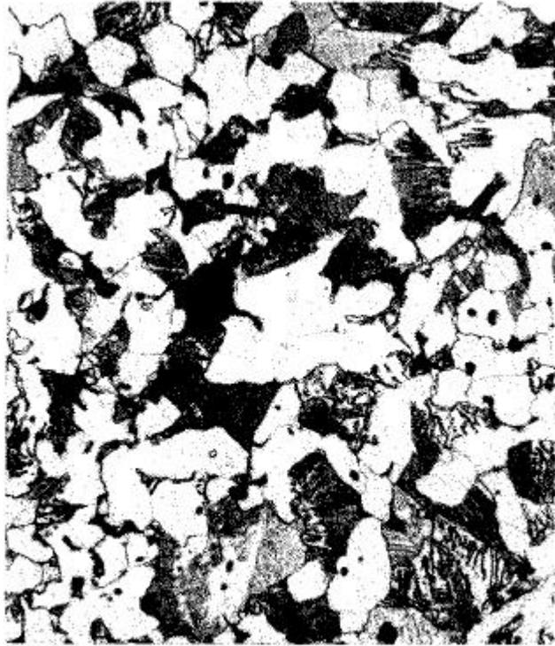
**Figure 1: As-sintered microstructure of FN-0205.**
