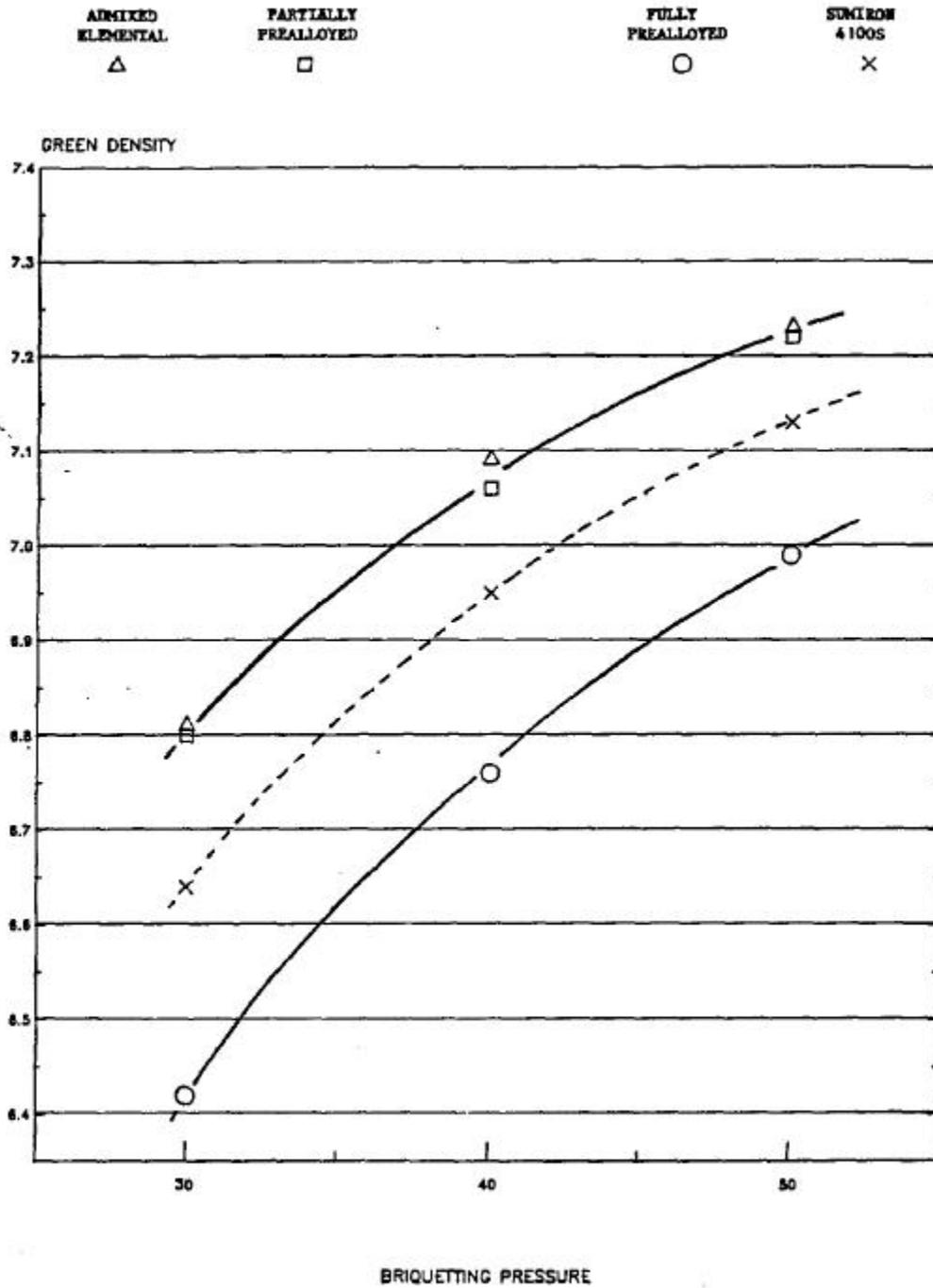
Figure 2: Compressibility curves for the various powders. (Each material contained 0.6 wt. % graphite and 0.5 wt. % Acrawax.)
