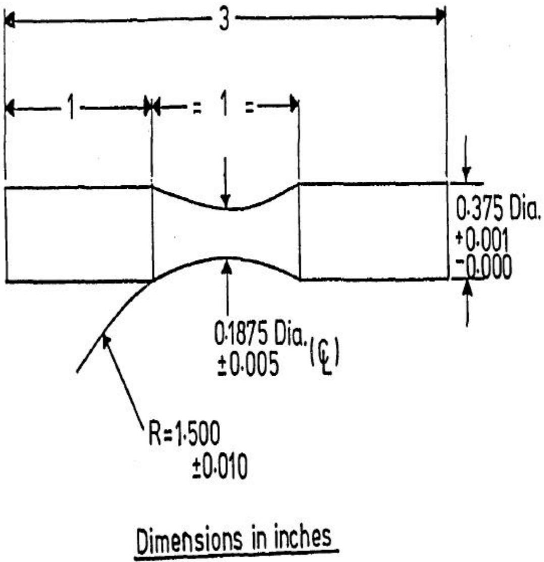
Figure 3: Rotating Bending Fatigue (RBF) Test Piece
