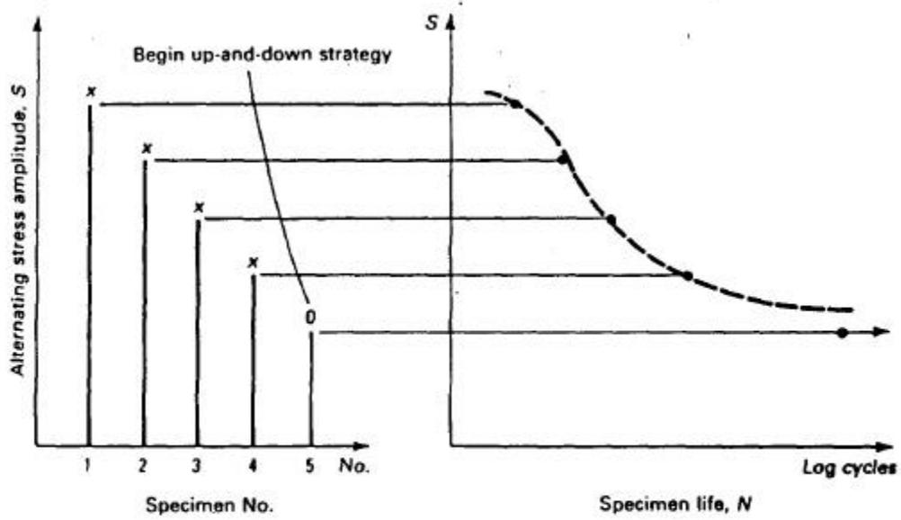
Figure 8: Schematic of  $S/N$  data generated as a preliminary test for subsequent two point program beginning with up and down strategy.
