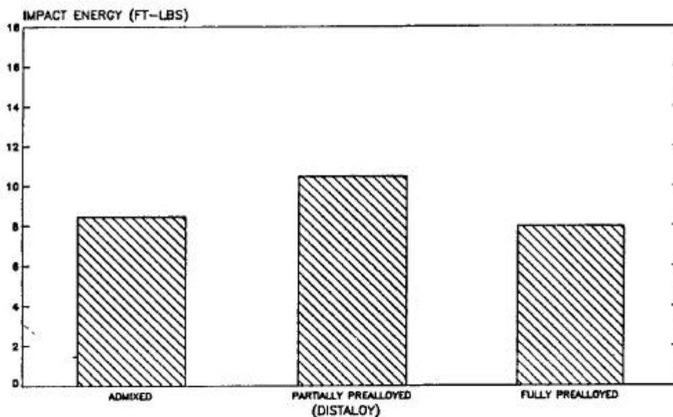
Figure 4: Room temperature unnotched Charpy impact energy data for samples pressed to a green density of 6.9 g/cm<sup>3</sup>. (Sintered in dissociated ammonia for 30 minutes at a temperature of 2050°F.)
