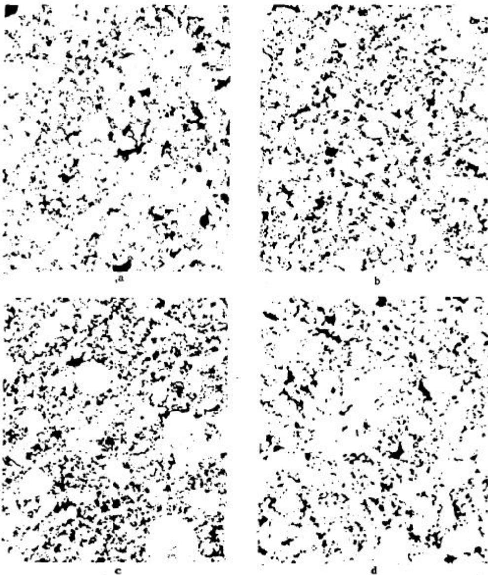
Figure 10: Photomicrographs of the unetched microstructures of the various samples: x100. (Samples compacted at 45 tsi and sintered at 2050°F for 30 minutes at temperature in a dissociated ammonia atmosphere - Sumiron 4100S sintered at 2300°F.)
