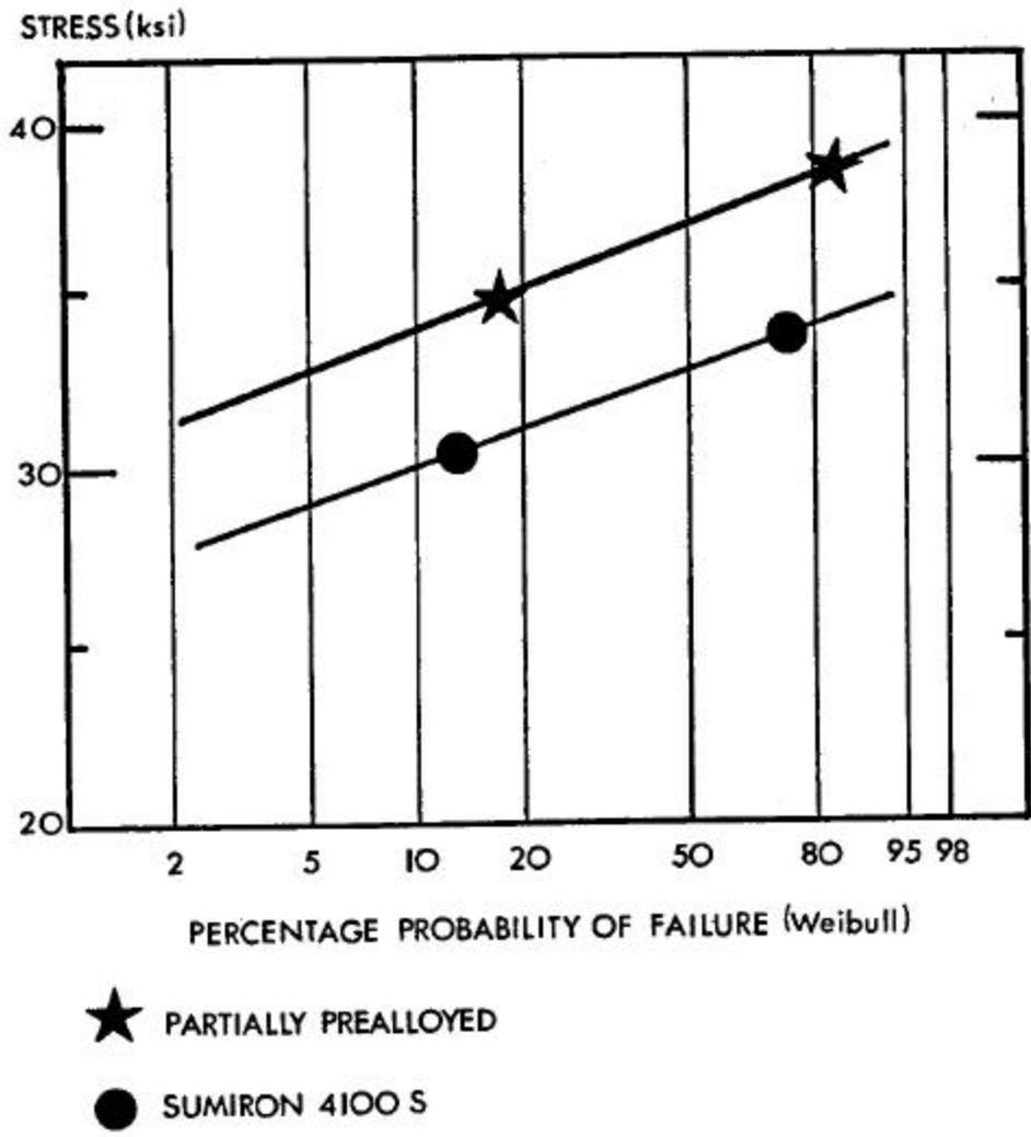
Figure 9: Stress versus the percentage probability of failure in rotating bending fatigue. (Samples compacted at 45 tsi and sintered for 30 minutes at temperature in a dissociated ammonia atmosphere. The partially prealloyed material was sintered at 2050°F and the Sumiron 4100S was sintered at 2300°F.)
