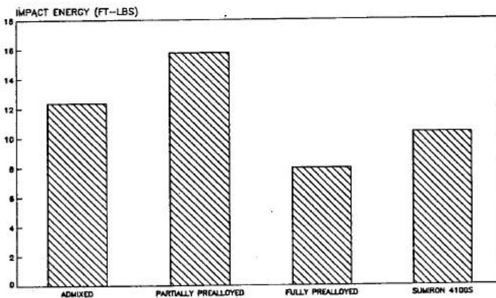
Figure 5: Room temperature unnotched Charpy impact energy data for samples compacted at 45 tsi. (Sintered in dissociated ammonia for 30 minutes at 2050°F - Sumiron 4100S, 30 minutes at 2300°F.)
