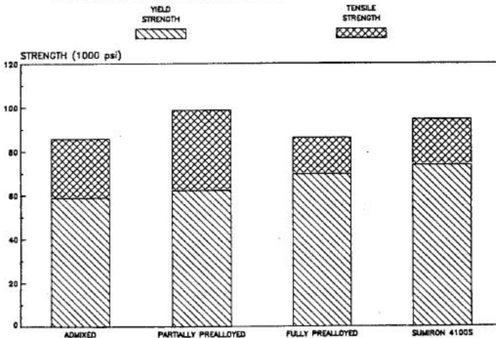
Figure 7: 0.2% offset yield strength ( $R_{p0.2}$ ) and UTS data ( $R_m$ ) for samples compacted at 45 tsi. (Sintered in dissociated ammonia for 30 minute at 2050°F - Sumiron 4100S, 30 minutes at 2300°F.)
