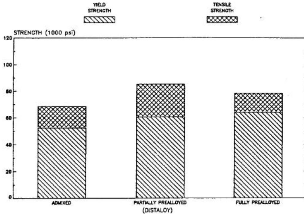
Figure 6: 0.2% offset yield strength ( $R_{p0.2}$ ) and UTS data ( $R_m$ ) for samples pressed to a green density of 6.9 g/cm<sup>3</sup>. (Sintered in dissociated ammonia for 30 minutes at 2050°F.)
