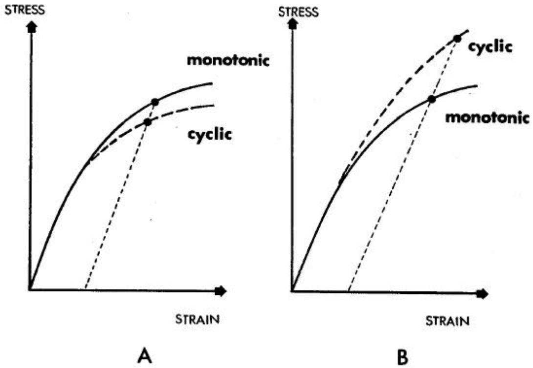
Figure 12: Monotonic and cyclic stress-strain curves.
