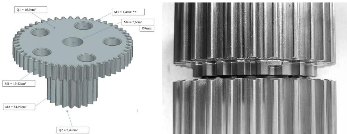
**Figure 7:** Parts from different compaction studies
