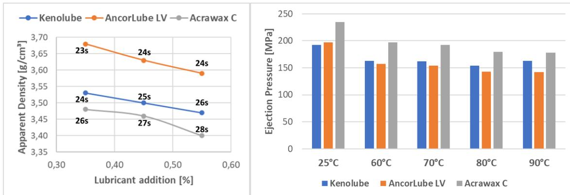
**Figure 4:** Apparent densities and Hall flows for different lubricant concentrations (left) as well as ejection pressures at five different tool temperatures after 700 MPa compaction (right) for material Ancorsteel 1000BMn + 1.5% Cu + 0.55% C as Ancorbond plus 0.35% lubricant added.
