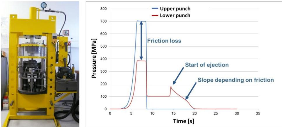
**Figure 2:** Instrumented press used for measuring compaction pressures (left) and typical compaction curve for a bushing (OD=14.3 mm, ID=9.0 mm, Height=15 mm) (right).
