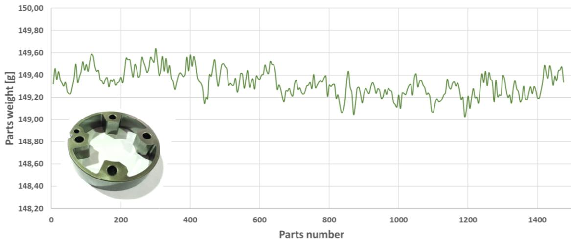
**Figure 6:** Compaction study of VVT stator components with Ancorsteel 1000BMn + 17% FD10Cu + 0.65% C + 0.6% AncorLube LV, press rate of 10 strokes per minute
