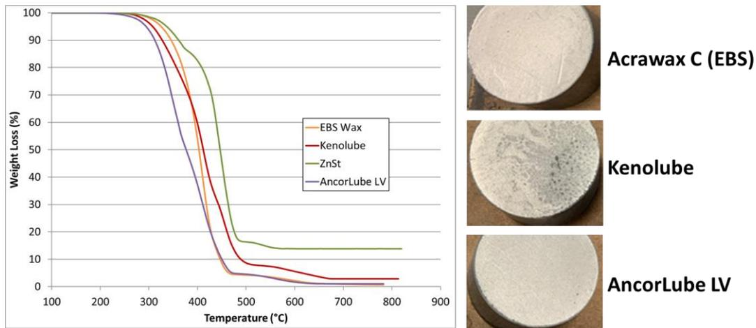
**Figure 5:** TGA-measurement of pure lubricant samples (left) and surface finish of cylinders made of Ancorsteel 1000 B + 2% Cu + 0.8% C + 0.6% lubricant sintered at 1120 °C in an atmosphere of 90%N<sub>2</sub>/10%H<sub>2</sub>
