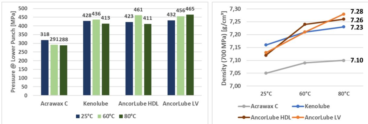
**Figure 3:** Lubricity measurements for 700 MPa of different lubricants (left) and compressibility at three different tool temperatures (right) for premix material Ancorsteel 1000 BMn + 1.5% Cu + 0.55% C + 0.5% lubricant.
