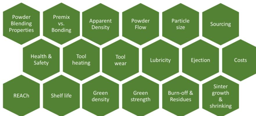
**Figure 1:** Key properties of modern PM lubricants.
