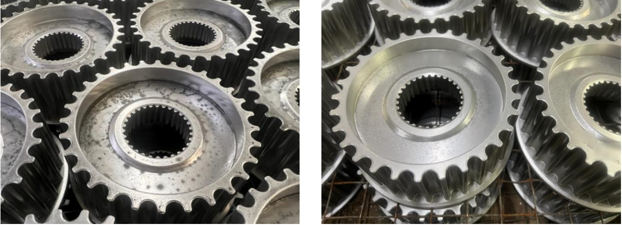
Figure 11: Sintered surface finish on standard production (left) and 0.55% AncorLube LV sample (right)
