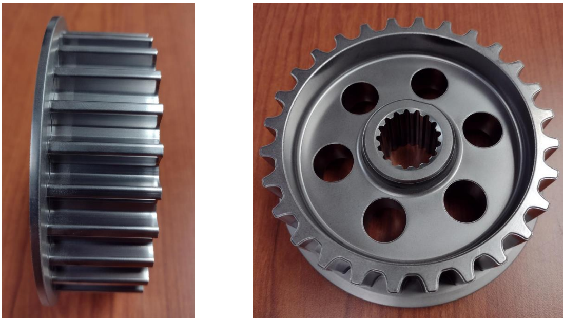
Figure 3: Sprocket geometry shown in die face view (left) and punch face view (right)
