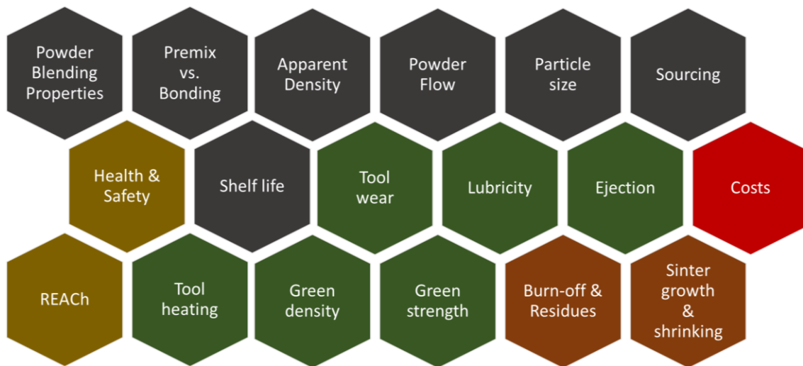
Figure 1: Essential properties needed in modern PM lubricants (colors reflect different process steps)
