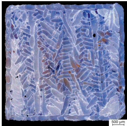
Figure 16: Cross section, overview. Light microscope, Kroll etchant. Segments of melt pools in multiple orientations from multiple build planes.
