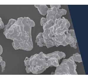
This is a water atomized, prealloyed steel powder specifically developed for sinter-hardening for a range of part sizes. The primary characteristics center on excellent hardenability in conjunction with good compressibility, particularly at higher compaction pressures. This unique combination of attributes differentiates its performance and optimizes both static and dynamic strength.
