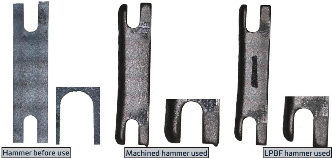
Standard screens wear more quickly (increasing hole diameter) and failed after ~1,150 kgs of Fe-Ti-Mn processed; LPBF screens still highly functional
