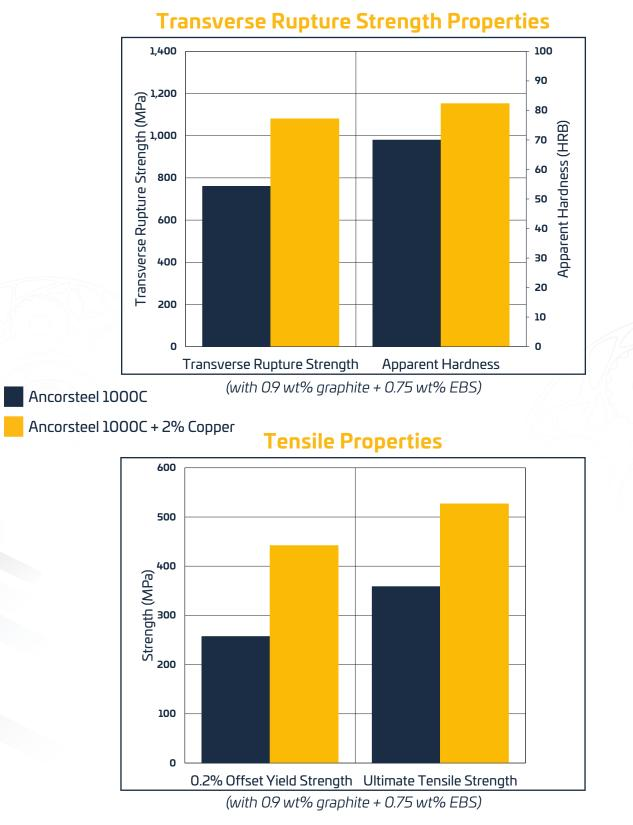
All test specimens were compacted to 7.0 g/cm<sup>3</sup> and sintered at 1120 °C (2050 °F) in  $90N_2$ -10H<sub>2</sub> atmosphere with conventional cooling.
