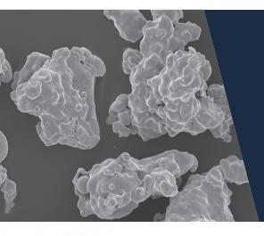
This is a water atomized, prealloyed steel powder specifically developed for sinter-hardening for a range of part sizes. The primary characteristics center on excellent hardenability in conjunction with good compressibility, particularly at higher compaction pressures. This unique combination of attributes differentiates its performance and optimizes both static and dynamic strength. This material conforms to MPIF standard 35 for FL-480X.
