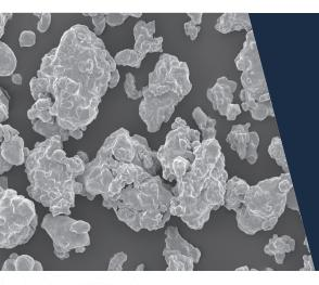
This is a water-atomized, prealloyed, low-alloy steel powder for high performance applications. The higher prealloyed 1.50 weight % molybdenum addition permits good compressibility as well as good response to heat treatment and sinter-hardening. This material conforms to MPIF standard 35 for FL-4905.
