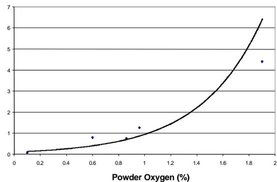
Figure 6 - Surface area versus Oxygen content.
