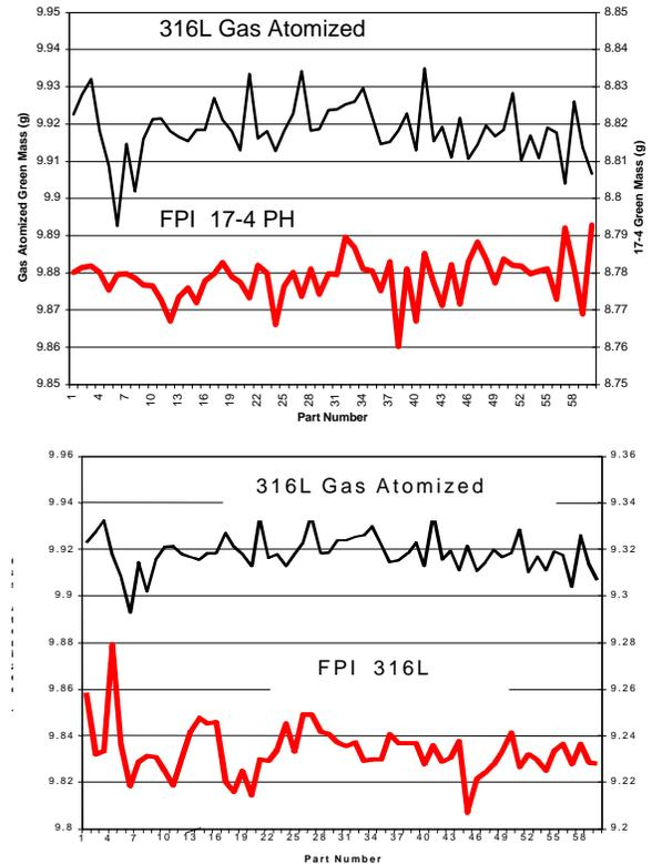
Figure 8a,b - Compares as-molded weight variation of gas atomized 316L to FPI 17-4 PH (top) and FPI 316L (btm).
