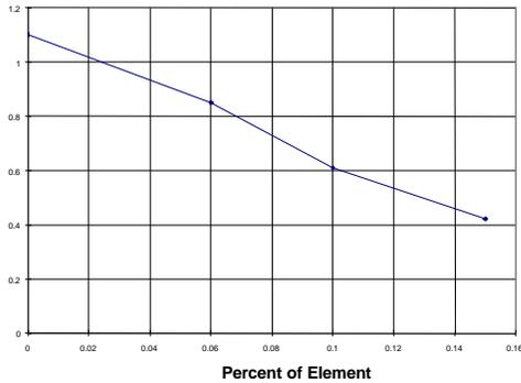
Figure 7 - Effect of oxide forming element on powder oxygen content
