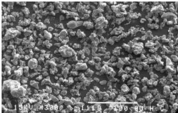
Figure 3 - Particle shape associated with typical water atomization process.
