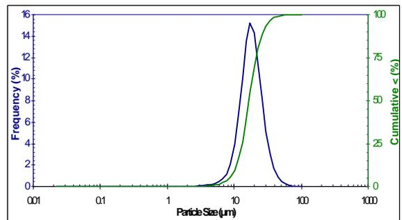
Figure 2 - Particle size distribution for 316L
