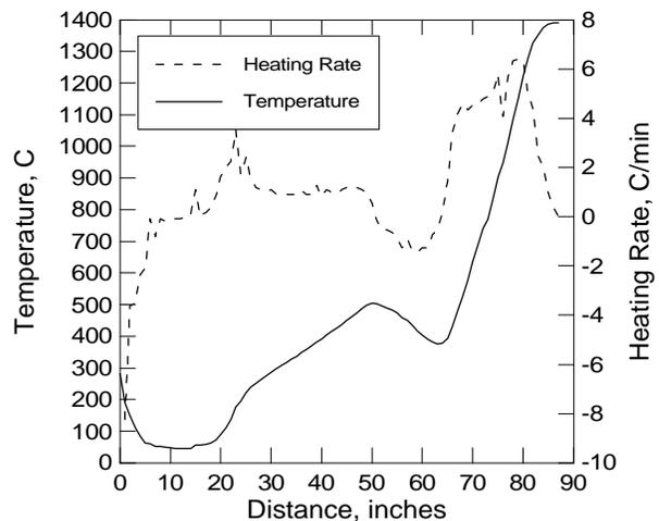
Figure 9 - Furnace profile for initial 316L sintering trial.
