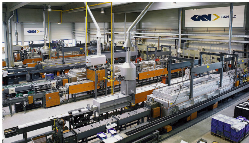
Fig. 1 A view of the continuous debinding and sintering facilities at GKN Sinter Metals' MIM operation in Bad Langensalza, one of the largest in Europe
