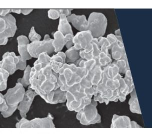
Ancorsteel DWP200 is a low apparent density water atomized powder for structural applications. The atomizing process imparts a more irregular spongy morrphology to the powder particles giving DWP200 a superior combination of green strength and compressibility compared to other atomized powders.
