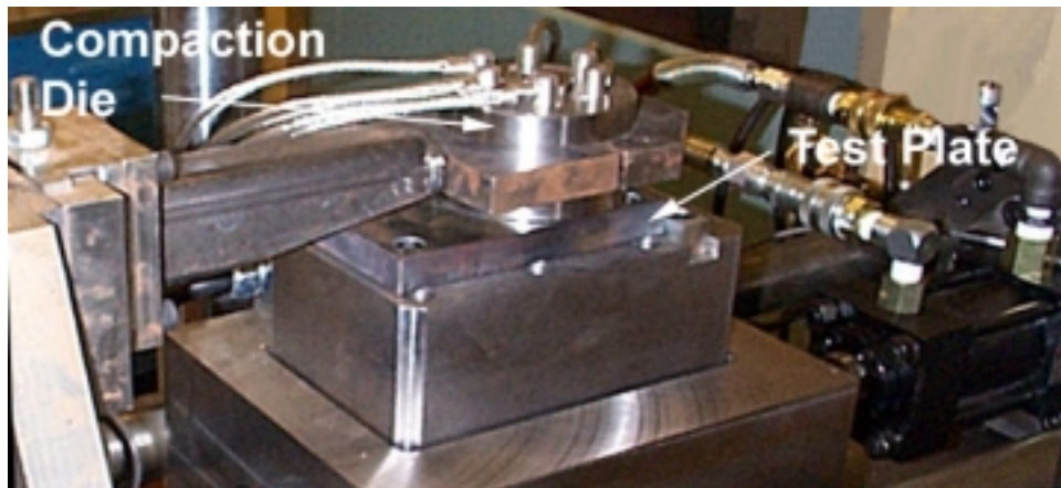
Figure 4. Caterpillar direct friction measurement device.
