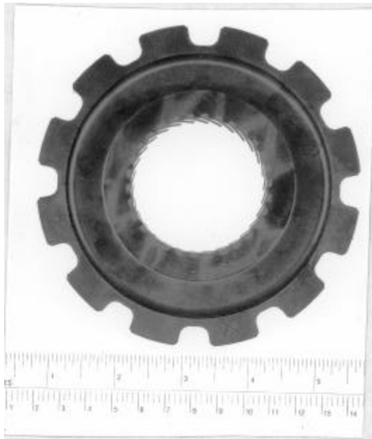
Fig. 2: P/M Transmission Parking Brake
